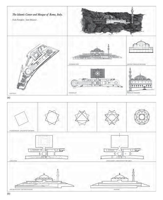
Figure 4.11 The Islamic Center of Rome: (a) formative concepts; (b) analytic diagrams. (Graphics by Raheel Ahmad; drawings by Latif Abdulmalik)
